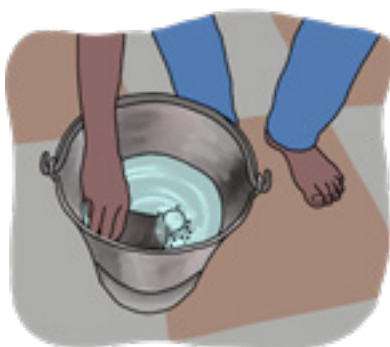
Fig. 1. Demonstrating that an empty tumbler contains air. An empty tumbler is inverted and immersed into water. When it is tilted slightly, students can see air bubbles escape from it and rise to the water surface.
