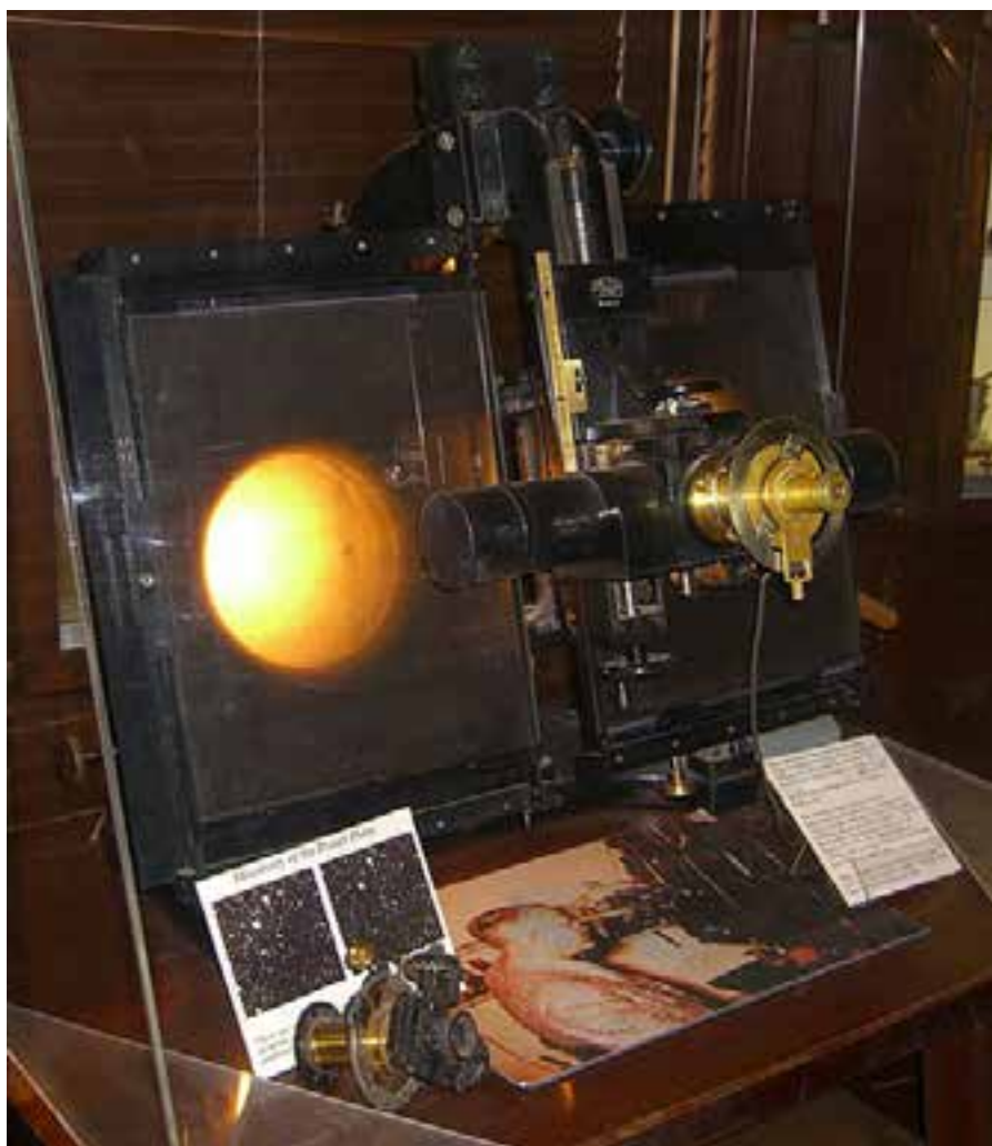
Fig. 1. A blink comparator. Lowell and Tombaugh sat in front of this instrument for hours, comparing photographs of the night sky for movements of Lowell's Planet X.
