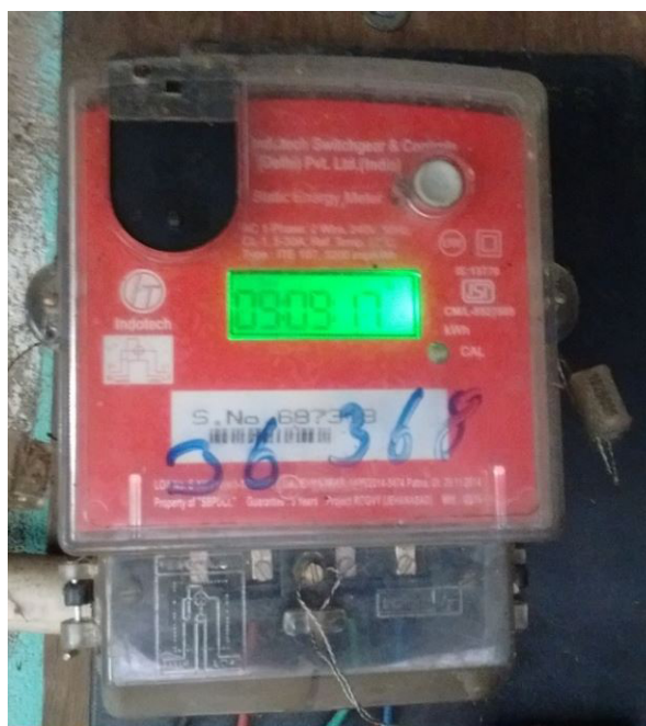
Image 2: The state electricity grid meter with variable readout of metrics that are difficult to understand.
