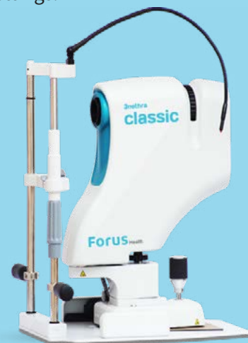
Figure 5.3: 3nethra classic: A digital imaging device that displays, stores, and transmits images of the posterior and anterior surfaces of the human eye
