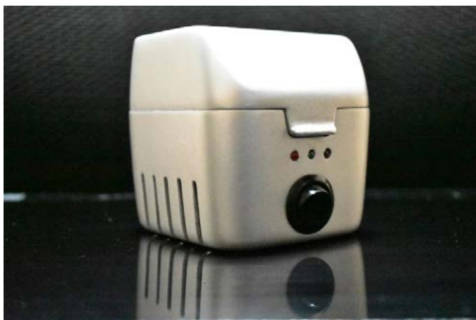
Figure 3.2 Amplicube, a portable isothermal device Source: https://www.agnii.gov.in/innovation/amplicube
