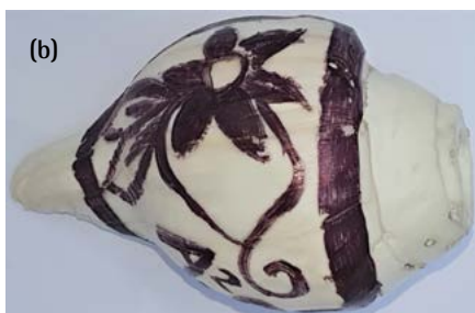
Fig. 3. The results of etching and anti-etching techniques. (a) A negative image of the crescent moon and stars. Here the background is painted with nail polish. Since this is hydrophobic, the acid solution reacts only with the exposed, unpainted surface. The moon and stars show depth. (b) A positive image of a flower. Since the flower areas are painted with nail polish, the acid solution will react only with the unpainted background. The flower will look elevated. Credits: Ranjit Kumar Dash. License: CC-BY-NC.
