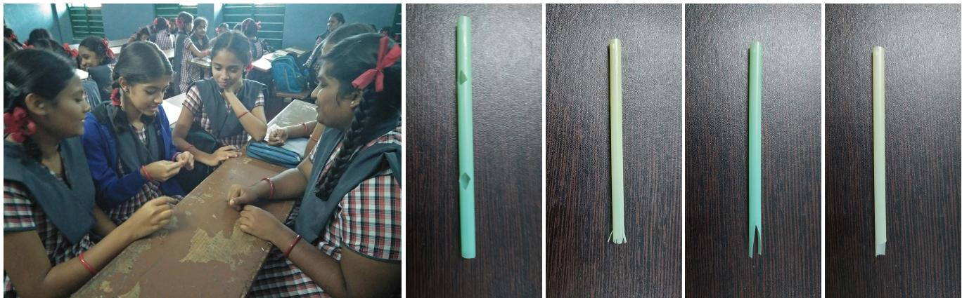
Students brainstorming on ways to modify their straws to produce sound. On the right are the different designs that students came up with, each producing varying levels of sound. The one that appears second last is the one that produced the loudest sound.
