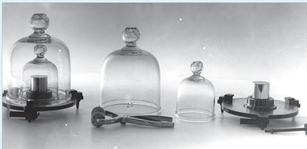
Le Grand K are used as national standards. The platinum-iridium cylinder to the extreme right is the copy (called Kilogram No. 20) used as the national standard of the kilogram in USA. The cylinder to the extreme left and under a bell jar (called Kilogram No. 4) is a duplicate of Kilogram No. 20 that is used as a secondary standard.
