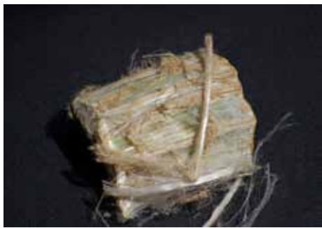
Figure 12a. Asbestos: fibres made of double stranded silicate chains. Source: Nikhil Fernandes.
