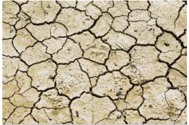
Figure 16. Soils containing expanding 2:1 clays crack and shrink when dry. Source: jackmac34, Pixabay. License: Public Domain. URL: https://pixabay.com/en/drought-earth-desert-aridity-711651/
