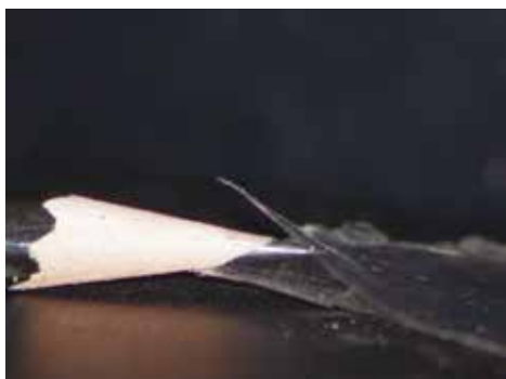
Figure 12b. Mica: made of sheets of silica tetrahedra. Source: Nikhil Fernandes.
