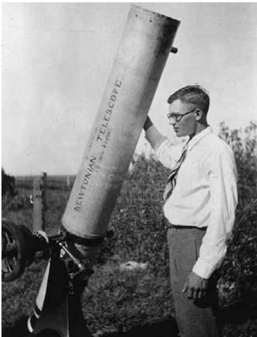
Fig. 2. Clyde Tombaugh with his homemade 9-inch telescope. He ground the mirrors for it himself. He also built his own mount with part of the crankshaft from his father's 1910 Buick (a car model) and discarded parts of a cream separator (used on his family's farm). This was the telescope that allowed him to observe markings on the surface of Jupiter and Mars.
